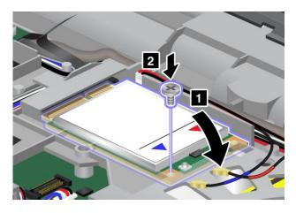
**Note:** Depending on the system configuration of your computer, the card might have only one connector. 10. Connect the cables to the new wireless WAN card.
